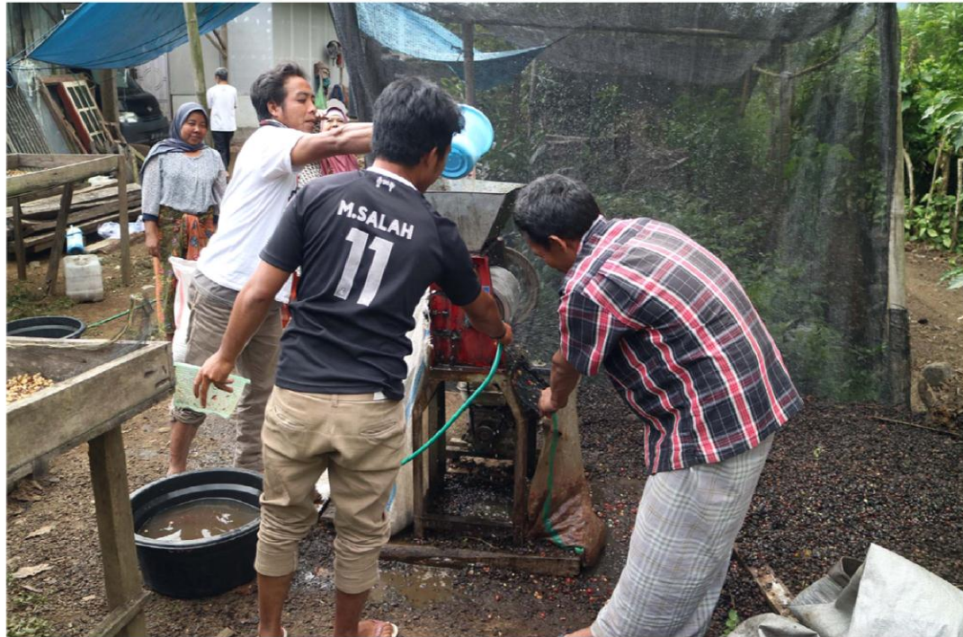
Pengolahan Buah Kopi : Pulpering (Proses Full Washed, Wet Hull dan Honey)
